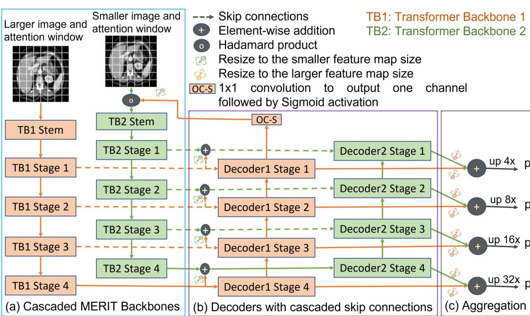
p1, p2, p3, and p4 are the aggregated multi-stage prediction maps. We can get the Parallel MERIT architecture by removing early feedback (through OC-S) from backbone 1 to backbone 2 and cascaded skip connections.
